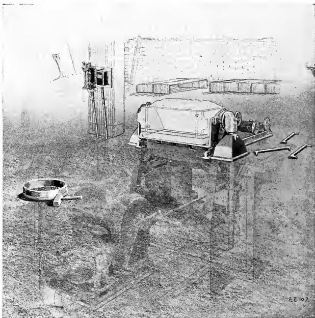
Fig. 152. Foundry Floor View of 42-inch Electrically Operated Roll-Over Jolt-Moulding Machine, showing Foundations in Phantom.
